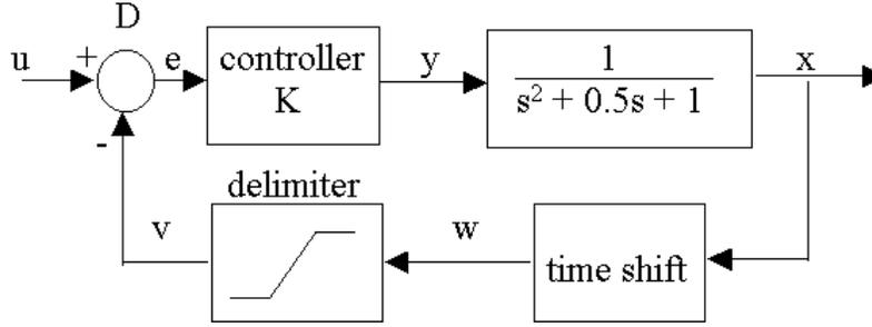
Figure 2. A control system with an ideal predictor.
