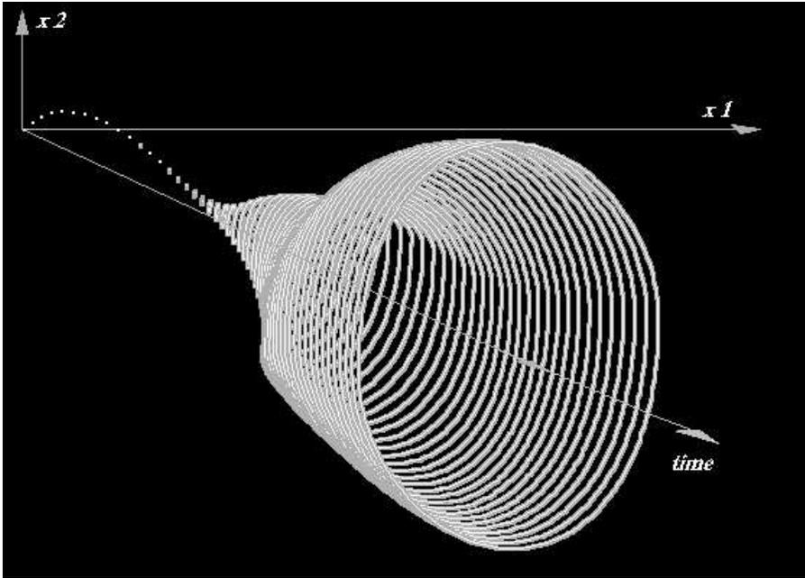
Figure 4. The reachable set for the system trajectories after iteration 14. The future uncertainty is taken from iteration 13.
